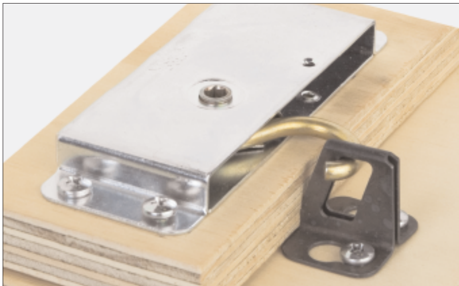
Fig. 2 The Big 'OT' Receiver is mounted to the face of a window frame, and is engaged by the spring hook of a large Type 1 Latch mounted on a thick hurricane panel. The slanted Receiver strike forces the Latch (and plywood) firmly against the window frame face, securing the panel against hurricane-force winds. This Big 'OT' Receiver will accommodate panel thicknesses from 1/4" to 3/4".
