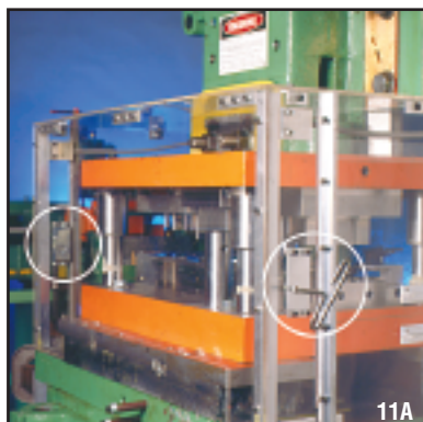
Fig. 11A & 11B Type 1R & 1L Latches and slot Receivers to quickly attach and remove machine guards, etc. Key operated for safety. (See TDS 23)
