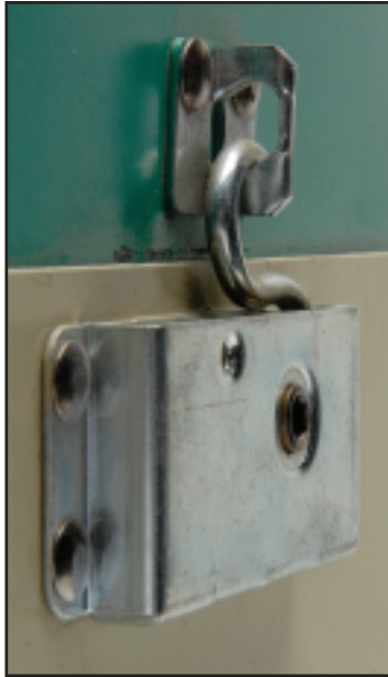
Fig. 1 In this view the 'OT' Receiver is mounted on the outside of the case and the Type 1 Latch is on the door, with the hinge below. The Latch hook pulling downward on the slanted surface of the Receiver forces the door inward against the case.
