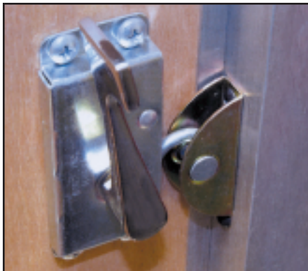
Fig. 1 Type 1 door Latch with handle using 'D' Receiver for 90° closure; both are surface mounted. Handle can be on opposite side. See TDS 17.
