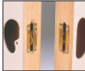
Fig 2A & 2B: The Type 3 Latch S1500-3-1.000 & Type 3 Receiver shown in these cutaway views of a flange-to-flange mounting in 3/4"/19mm thick framing places the access hole behind the frame.
