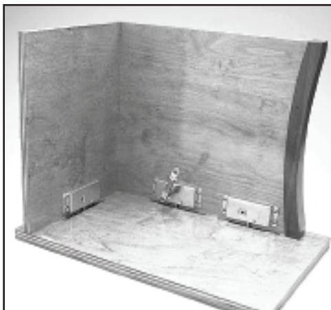
Fig. 1 A church pew section is shown here with surface mounted Type 1R Latches and flush mounted Type 2 RSL Receivers. These quick operating Latches facilitate attachment and removal of the seats for maintenance or recreational use of the floor area.
