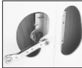
Fig 2A & 2B: The Type 3 Latch S1500-3-1.000 & Type 3 Receiver shown in these cutaway views of a flange-to-flange mounting in 3/4"/19mm thick framing places the access hole behind the frame.
