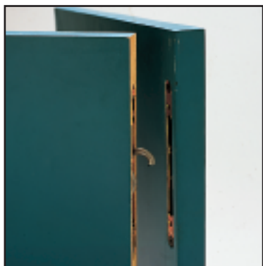
Fig. 1 Short Type 2 R/S Receivers require only a shallow (3/4" / 19mm deep) 'blind' mortise, facilitating fabrication of thin partitioning. This Latch/Receiver combination is used for in-line butt joints and for 'T' and corner joints.
