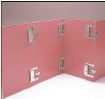
Fig. 8D Type 1R Latch with spring fingers and 'PL' Receiver for holding outside corners tight and at 90°. (See TDS 40)
