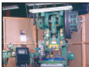
21. Acoustical Barrier Wall-Quickly Erected or Moved. Type 1, Type 2 or Type 3 Latch (see TDSs 36, 81 & 106).
