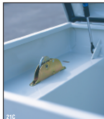
Fig. 21C Type 2 Latch for tool box security hold down onto a pick-up truck tray. (See TDS 81-2B, Fig 8 & TDS 92)
