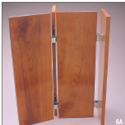
Fig. 6A, 6B, 6C For infinitely variable angled assemblies Type 2S Small Latches mounted in thin panels are joined here to 'O' and 'OD' Receivers in free standing and wall couplings. two, three, or more elements can be so connected. (See TDS 74)
