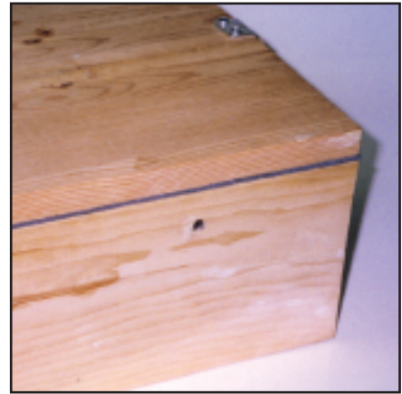
Fig. 3 The closed box shows only a hole for access to the Latch.
