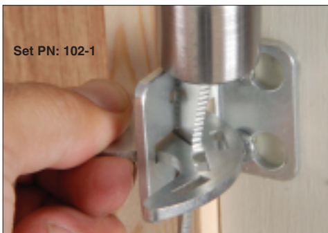
Fig. 4 PLYWOOD IS CLAMPED DOWN INSIDE WINDOW FRAME. HARDWARE IS ON FRAME FACE. NO "KEEPER" USED. PERMANENT HARDWARE IS 2 SCREWS. SEE TDS 206-3B.
