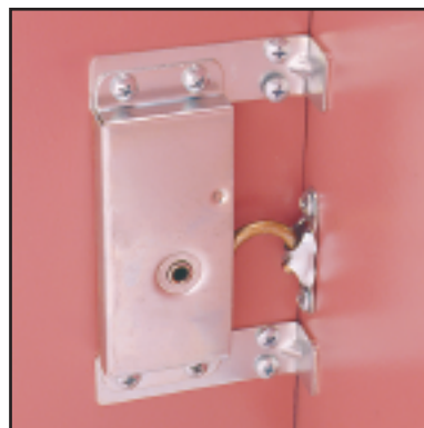
Fig. 5 A Type 1 Latch with braces and a 'U' Receiver hold wall panels tight in a 90° corner joint.
