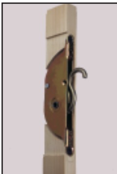
Fig. 4A & 4B The unique 'Taco' shape of the Type 2 Latches was designed to fit a straight-in/straight-out shaper cut for mortising expediency as seen in the cut away photos above. (See TDS 82)
