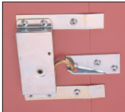
Fig. 8B Type 1R Latch with spring fingers and 'P' Receiver for keeping inline butt joints straight and tight. (See TDS 40)
