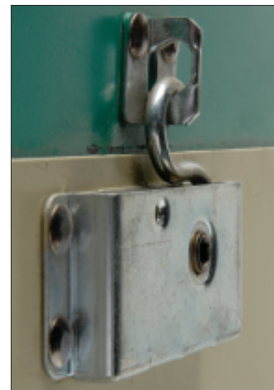
Fig. 4 In this view the 'OT' Receiver is mounted on the outside of the case and the Type 1 Latch is on the door panel, with the hinge below. The Latch hook pulling downward on the slanted surface of the Receiver forces the panel inward against the case.
