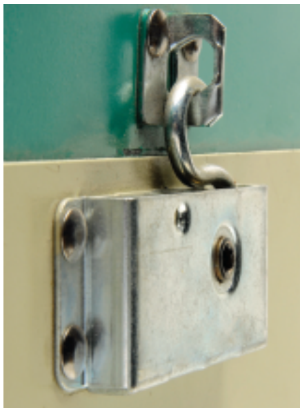
Fig. 1 In this view, the 'OT' Receiver is mounted on the outside of the case and the Type 1 Latch is on the door, with the hinge below. The latch hook pulling downward on the slanted surface of the Receiver forces the door inward against the case.
