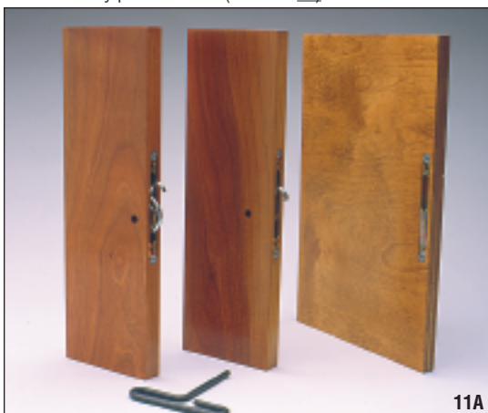
Fig. 11A, 11B Thin panels are shown here connected at butt and corner joints using Type 2 Latches and Receivers and the very shallow 'RSL' Receivers. Mortise does not break through the panel ('blind' mortise). (See TDS 62 & 66)
