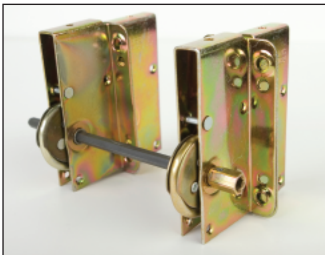
Fig. 3 “Ganged” Latches (two or more) using a shaft with an integral hex sleeve inserted thru the access hole after the panel is fabricated. Operation is by a hex key. See TDS 118-3 .
