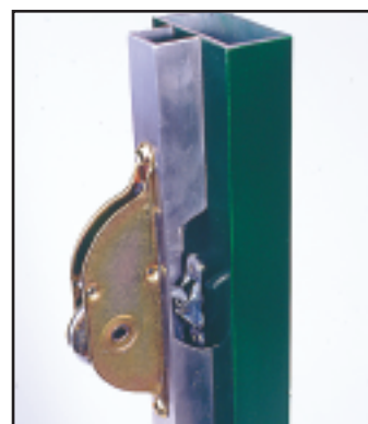
Fig. 9 A Type 2 Latch with a 'U' Receiver is shown above in a typical door or other style-to-frame joint. (See TDS 85)
