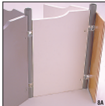
Fig. 8A, 8B, & 8C Type 2 Latches with 'CR' (Cup) Receivers and with 'T' brackets are used for infinitely variable angle free standing panel connections and also for variable angle connections to walls. (See TDS 94)
