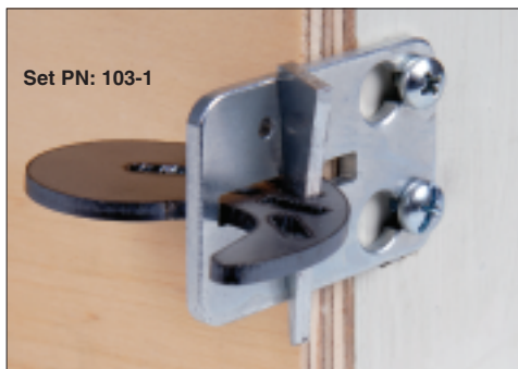
Fig. 5 PLYWOOD IS CLAMPED DOWN AGAINST WINDOW FRAME FACE. HARDWARE IS ON OUTSIDE WINDOW FRAME. PERMANENT HARDWARE IS 2 SCREWS. SEE TDS 206-4A.
