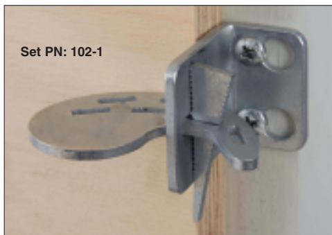
Fig. 3 PLYWOOD IS CLAMPED DOWN AGAINST WINDOW FRAME FACE. NO "KEEPER" IS USED. PERMANENT HARDWARE IS 2 SCREWS. SEE TDS 206-3A.
