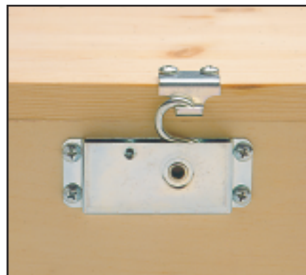
Fig. 15 Type 1R Latch and a 'JL' Receiver 'over the top' box closure application. (See TDS 19)
