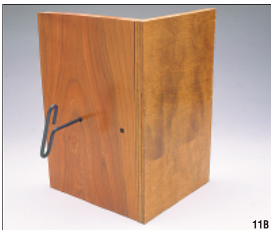
Fig. 11A, 11B Thin panels are shown here connected at butt and corner joints using Type 2 Latches and Receivers and the very shallow 'RSL' Receivers. Mortise does not break through the panel ('blind' mortise). (See TDS 62 & 66)
