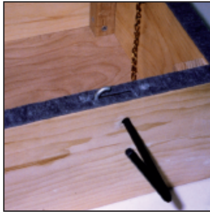
Fig. 2 Here, gasketing has been installed. The Latch operates through a slit.
