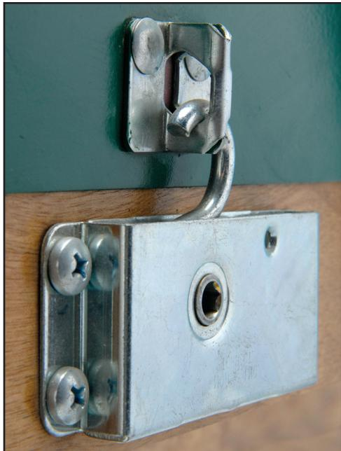
**Fig. 1** This is a view of an 'IT' Receiver mounted inside a case. The door is hinged outside from below. The Latch hook pulling against the slanted surface of the Receiver forces the door inward against the case. The Latch can be operated thru the door and sealed if required.
