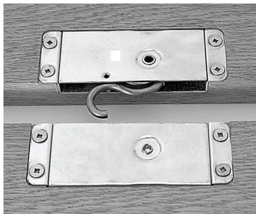
**Fig. 1** The Type 1R Latch and Receiver are shown in the unlocked condition, flush mounted underneath the flooring.
